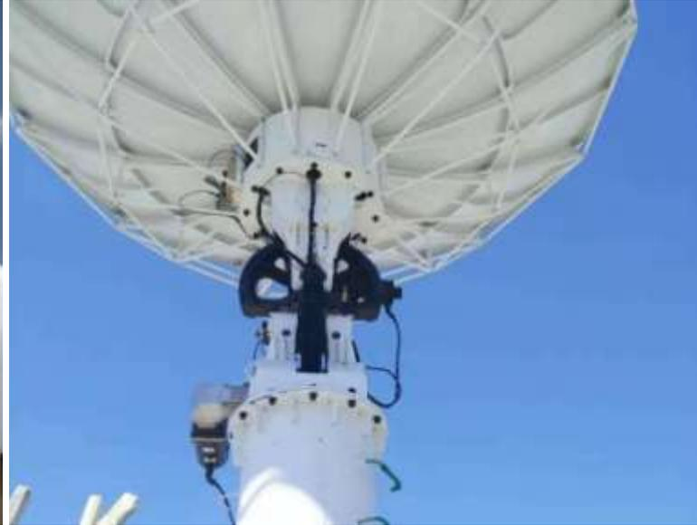
ATS- series antenna consists of 5.3/4.5/3.7 meters of dual reflectors or prime focus dish with X-Y pedestal configuration. The pedestal is mounted on a rigid base extension tube suitable for installation on ground, rooftop or on track with an optional NPM (None penetrating Mount). Thanks to dual shape optics for achieved the superior G/T performance and prime focus shape to be suitable for verity of application.
